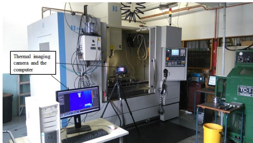
Figure 3.3: Bridgeport GX 1000 showing the machining setup.
