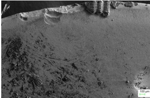
Figure 4.32: Failure mechanisms experienced by the uncoated ion implanted inserts.
