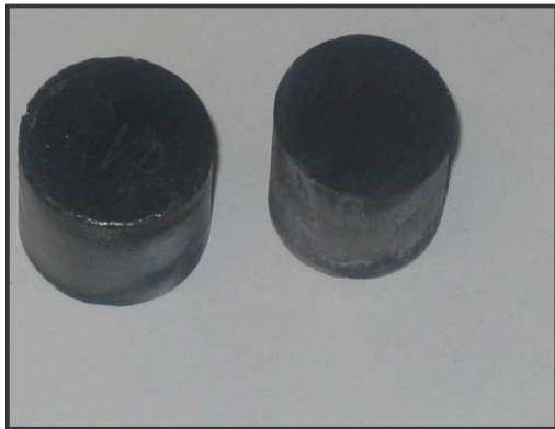
Fig. 4.36: Photographic image of alumina-cBN gelcasts sintered in argon at 1450°C for 3 hours.
