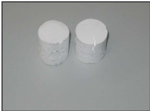
Fig. 4.37: Photographic image of alumina-cBN gelcasts sintered in air at 1450°C for 3 hours.
