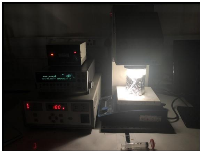
Figure 3.2: Image showing solar simulator and photocatalysis setup.
