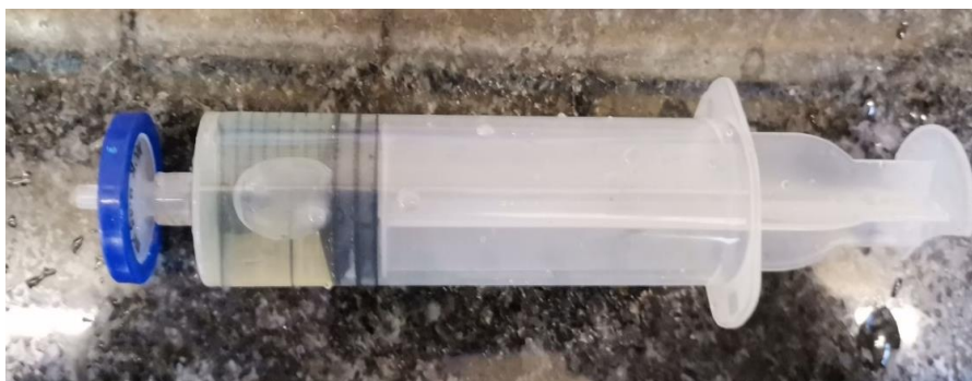
Figure 3-3: Image of the microfilter-syringe employed for leachate extractions.
