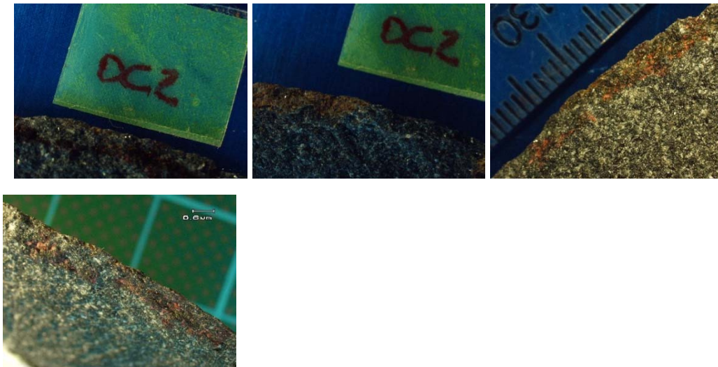
Top left, ventral surface before use; top centre, dorsal surface before use; top right, damage after 5minutes; bottom left, damage after 10 minutes.
