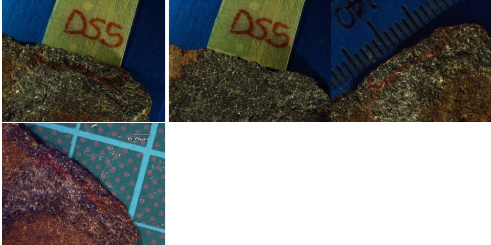
Top left, ventral surface before use; top centre, dorsal surface before use; top right, damage after 5minutes; bottom left, damage after 10 minutes.
