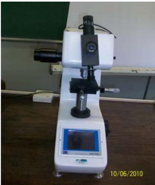
Figure 3.5: Vickers Micro hardness tester
