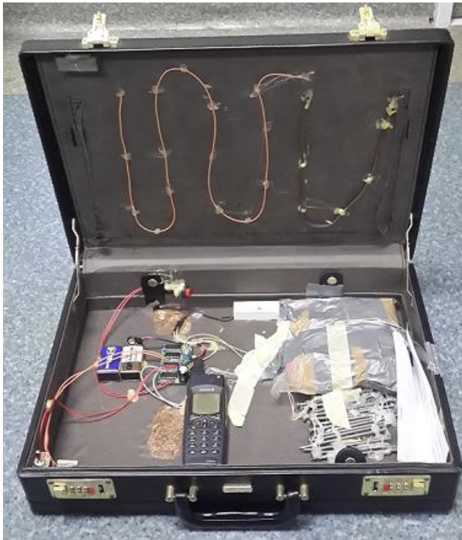
Figure 6: An image of the dummy IED built at the CSIR.
