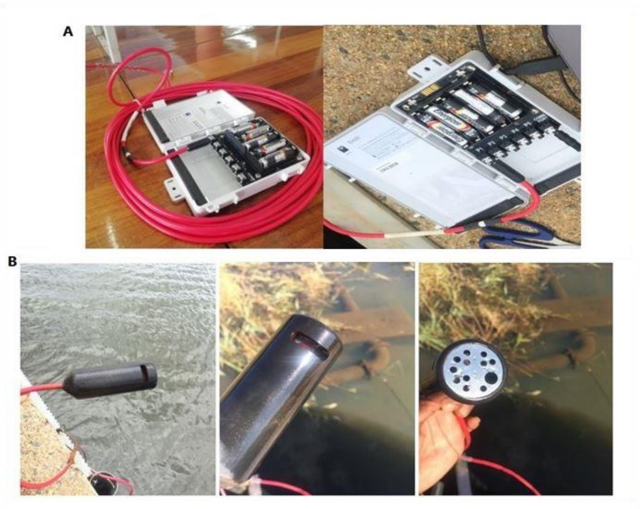
Figure 4: Equipment deployed for automated water quality observation network at the Sabi-Sand catchment. Panel A is the Em50 data logger powered with AA alkaline batteries and connected to a red 5 m submersible cable. Panel B is the Water Depth, Electrical Conductivity (EC), and Temperature CTD sensors—demonstrating the sensor’s full view, close-up view with the slight view of the inner electrodes and the front-top view as an inlet (stainless steel plate).
