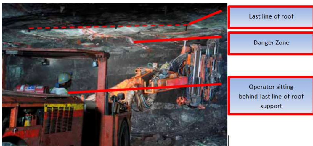
Figure 3.2: Danger-zone Indication: Typical (Sandvik, 2015)
