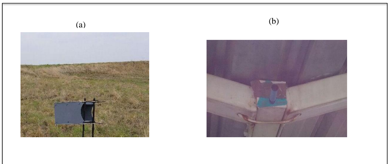
Figure 3.4: Picture of the passive samples at various locations in the South African International Airport. (a) Sample with a plastic shield covering; (b) Diffusive sampler on the triangle. Source: images were taken by the author.
