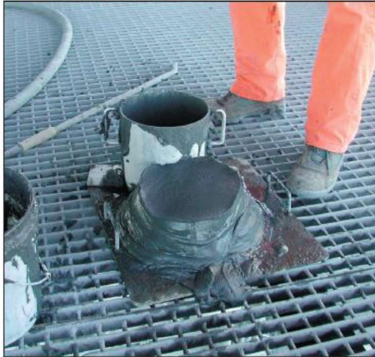
Figure 2-13: Cylindrical Slump Test (Grice, 2005)
