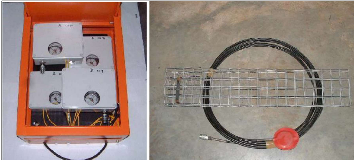
Figure 2-15: Components of the instrument used to measure backfill stress underground
