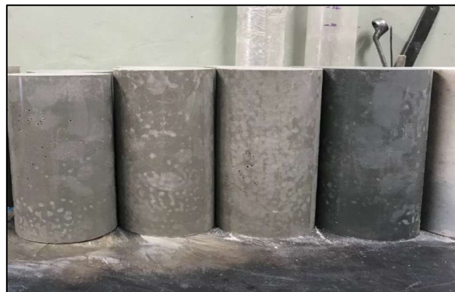
Figure 3-8: Backfill specimen after sample preparation.
