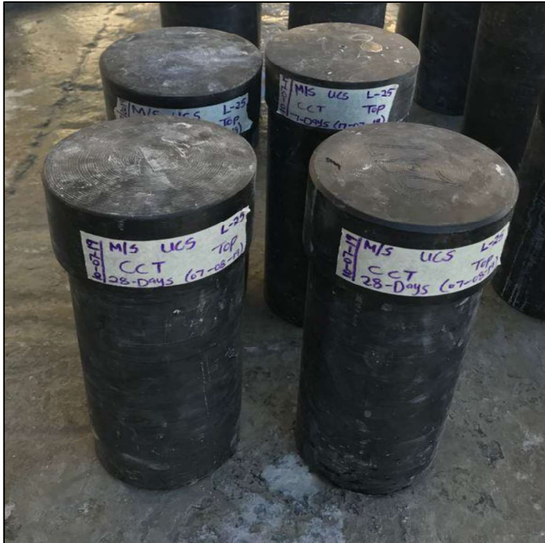
Figure 3-4: Backfill sample inside the PVC casings
