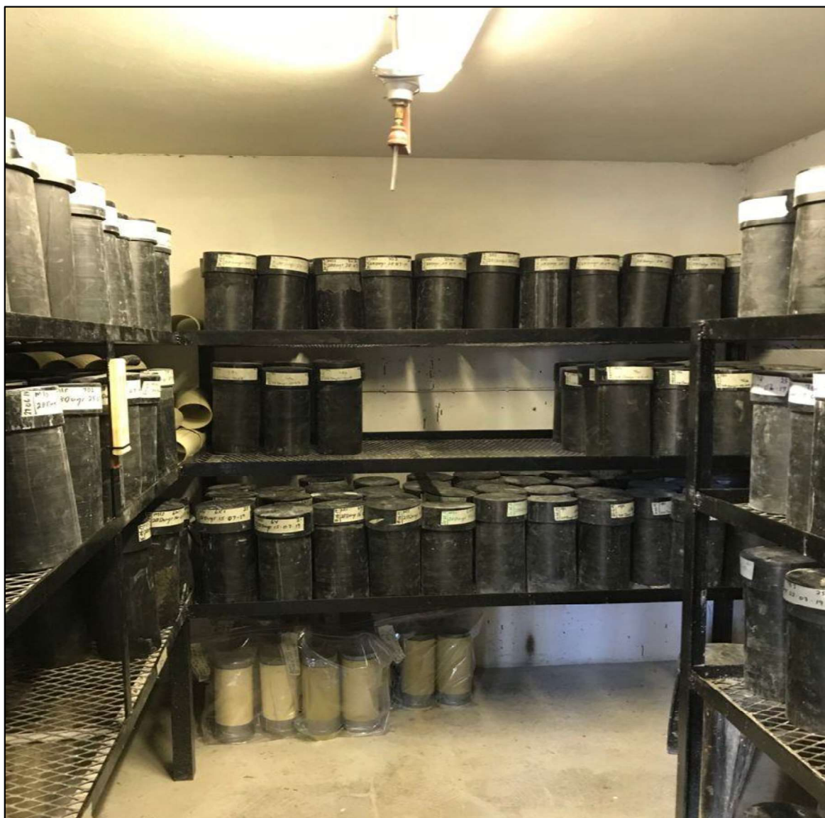
Figure 3-7: Backfill samples stored in the curing room
