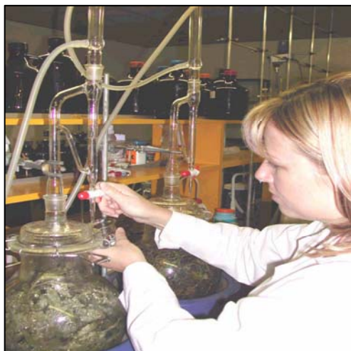
Figure 1: Process of hydrodistillation.
