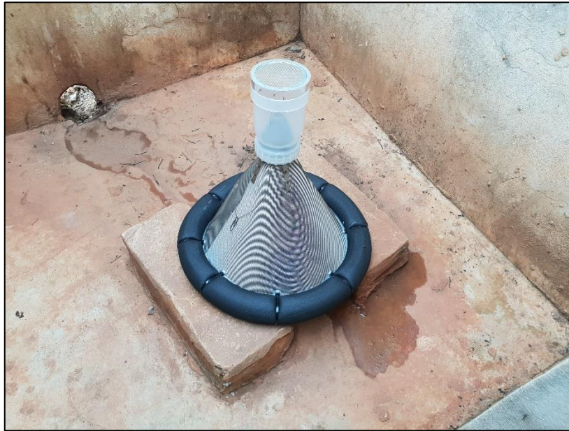
Figure 2.4. Hamer Emergence trap with 500ml collection jar, placed over a pit toilet.
