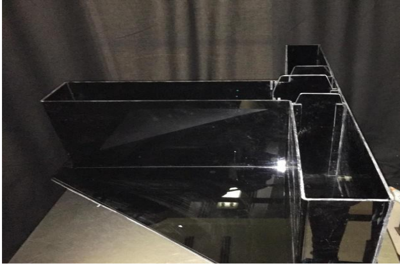
Figure 3. 17. T-Maze showing the characteristic three arms, made of black Perspex material.
