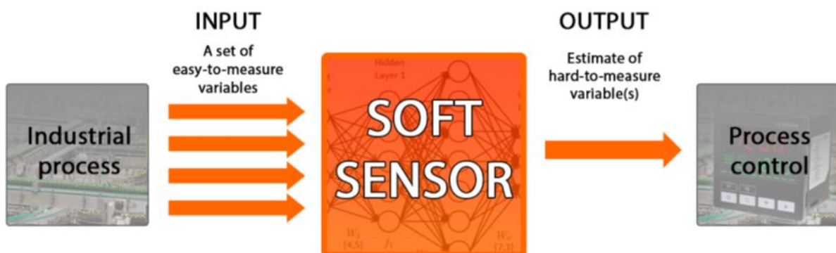
Figure 6: Working principle of a Soft Sensor (Curreri et al, 2020).
