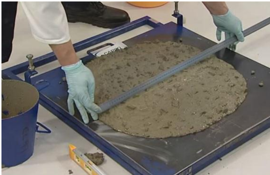
Figure 14: Slump measurement (Daily Civil, 2022).
