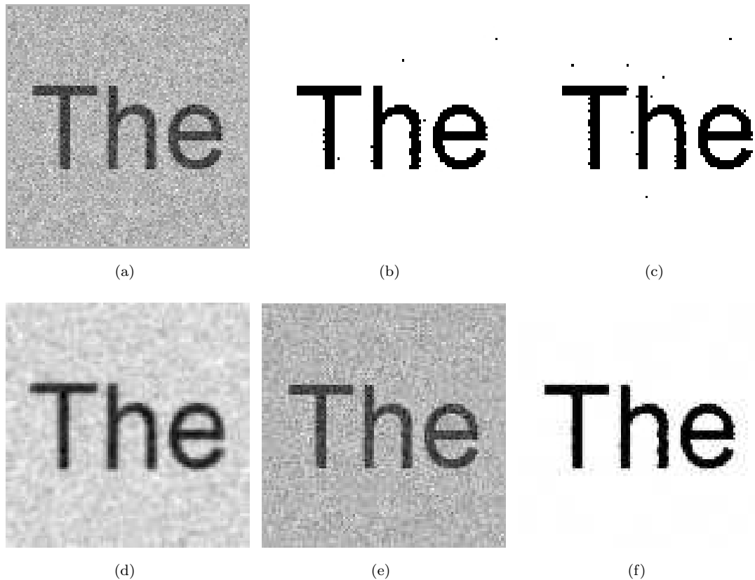
FIGURE 3.5: Binarization of an (a) initial noisy text sample, (b) result of Otsu's method, (c) result of Sauvola's method, (d) result of Linear Diffusion method, (e) result of Perona-Malik method and (f) our result.
