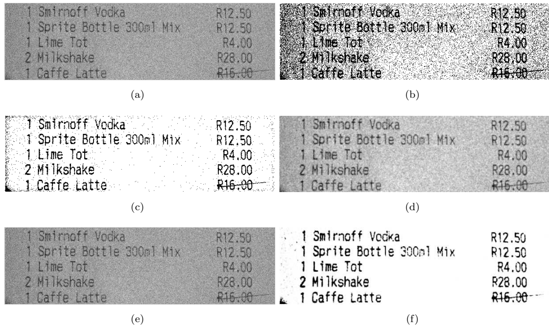
FIGURE 3.7: Binarization of an (a) initial noisy restaurant bill, (b) result of Otsu's method, (c) result of Sauvola's method, (d) result of Linear Diffusion method, (e) result of Perona-Malik method and (f) our result.
