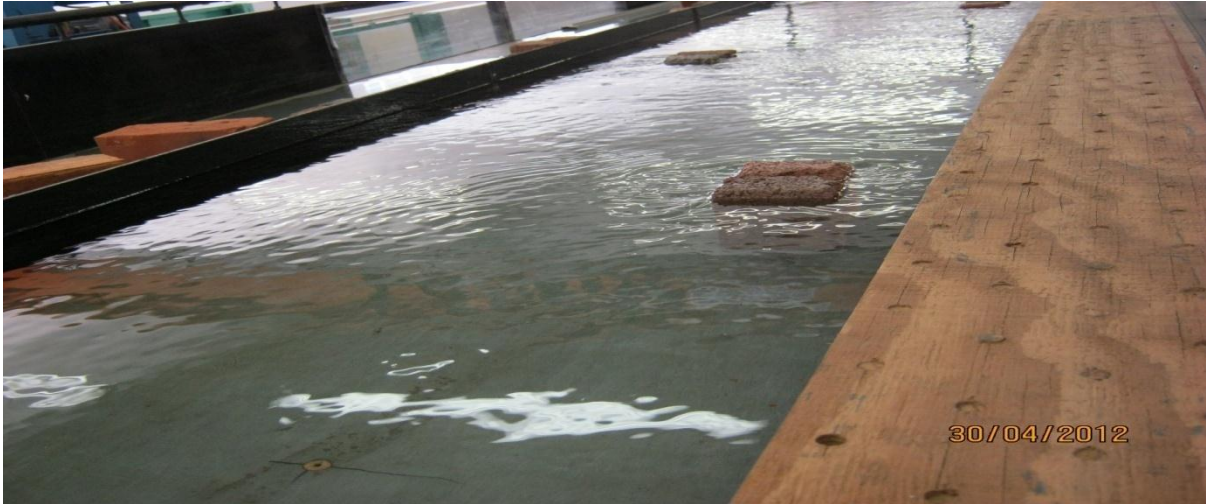
Figure A11. Smooth bed flume with combination of obstructions and vegetation.
