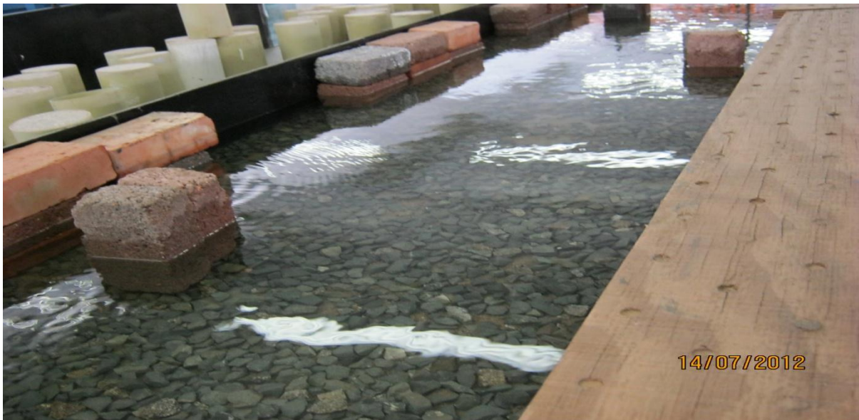
Figure A29. Rough bed flume with a combination of irregularities, obstruction and vegetation.
