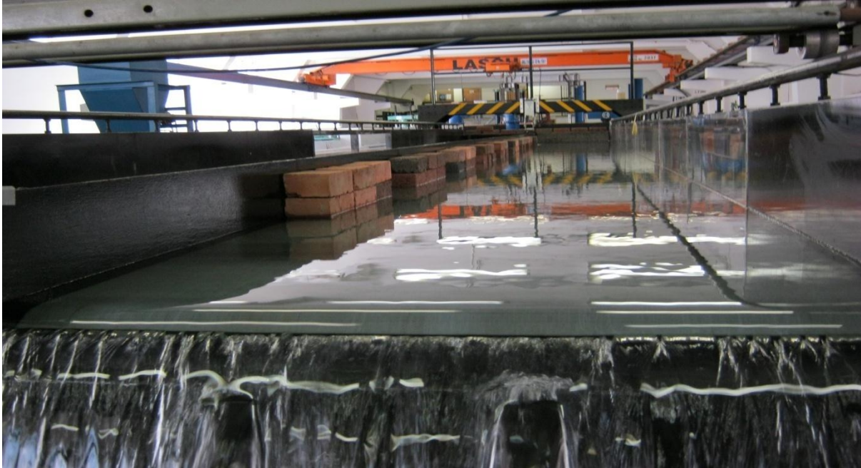
Figure A1. Smooth bed flume with irregularities.
