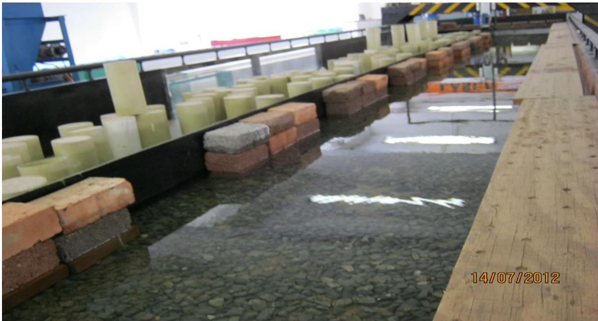
Figure A25. Rough bed flume with irregularities and vegetation.
