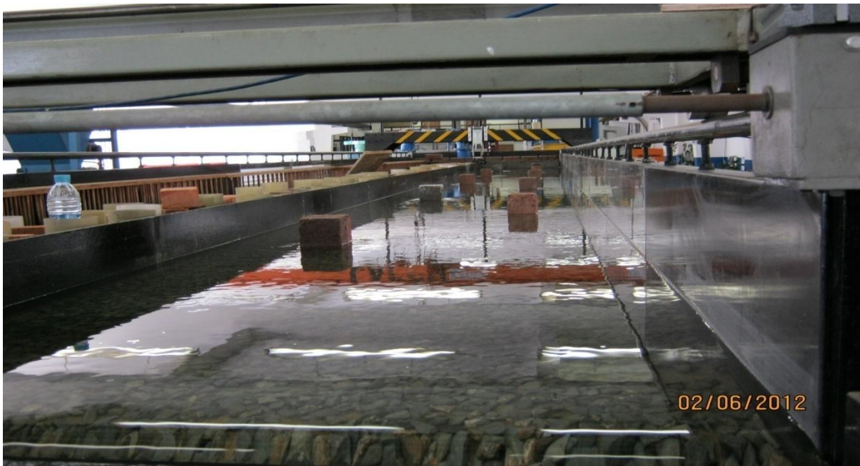
Figure A19. Rough bed flume with obstructions.
