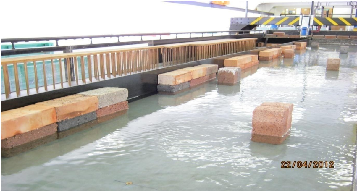
Figure A7. Smooth bed flume with irregularities and obstructions.
