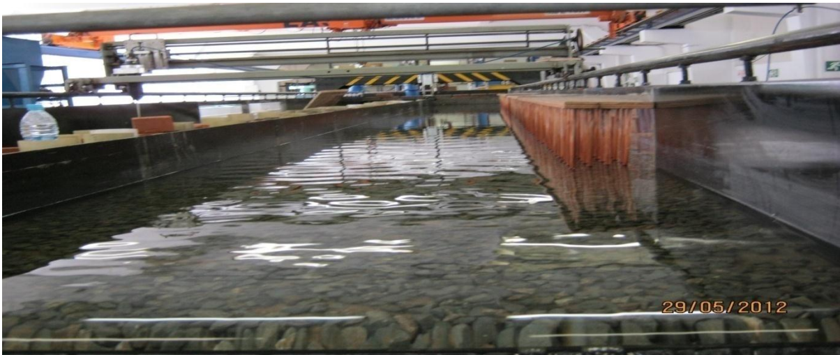
Figure A21. Rough bed flume with vegetation.
