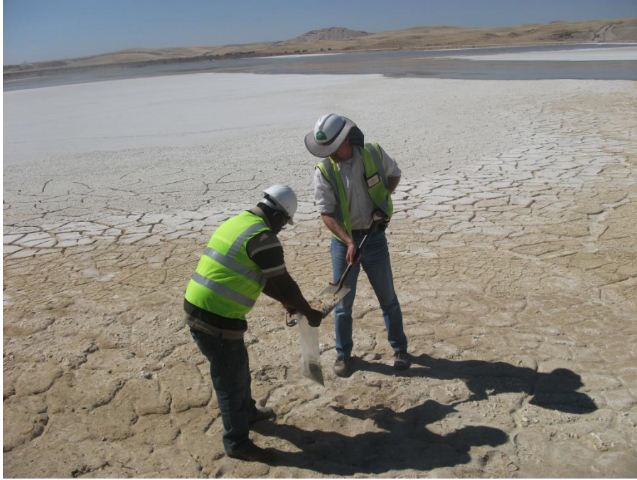
Figure 5. The author collecting soil samples on the unlined tailing facility at Langerheinrich mine in 2011, in the background are ponds of polluted water allowed to seep through the tailings
