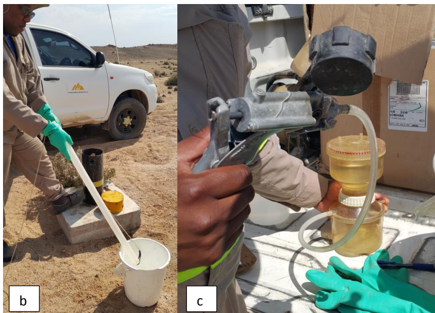
Figure 23. (a) The MP1 water sampling pump mounted on trailer (b) The water bailer, being used by the mine staff member (c) The filtering set used to filter water samples
