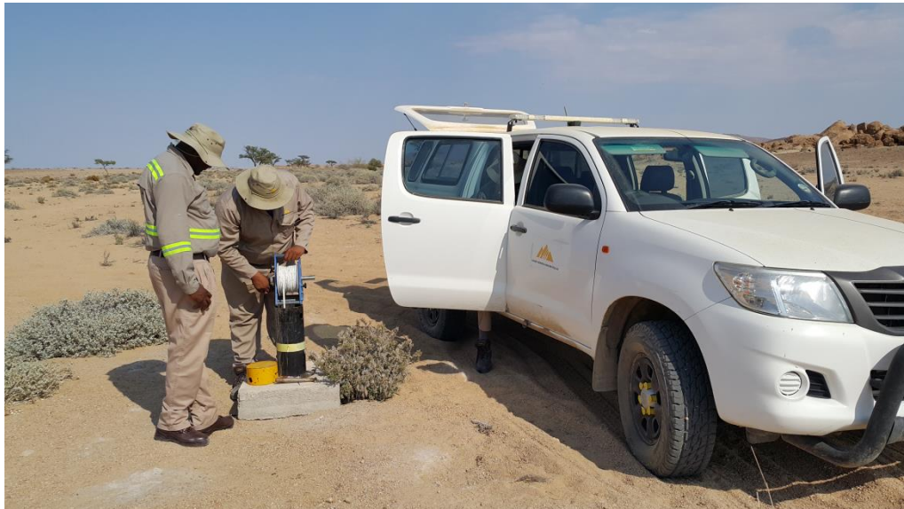
Figure 24. The dip meter used in the measurement
