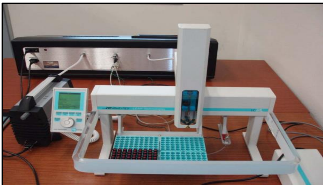
Figure 27. Liquid Water Isotope Analyser used for the analysis of oxygen-18 and deuterium
