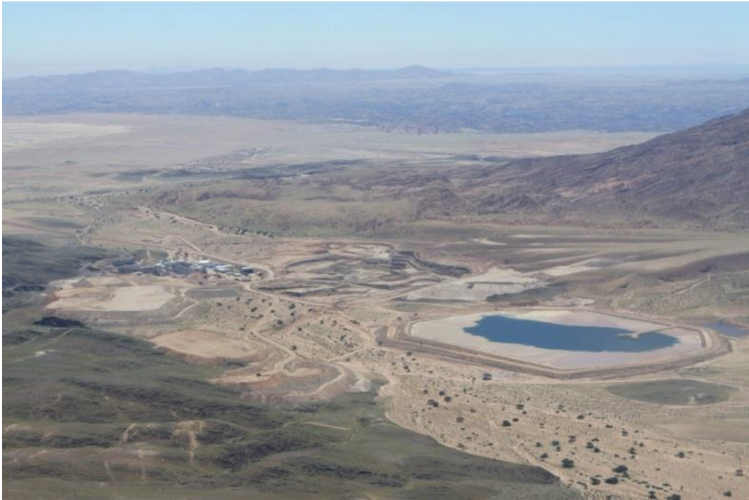
Figure 2. The aerial view of the Langerheinrich tailings on top of the Gawib River (Source: MME, 2010)
