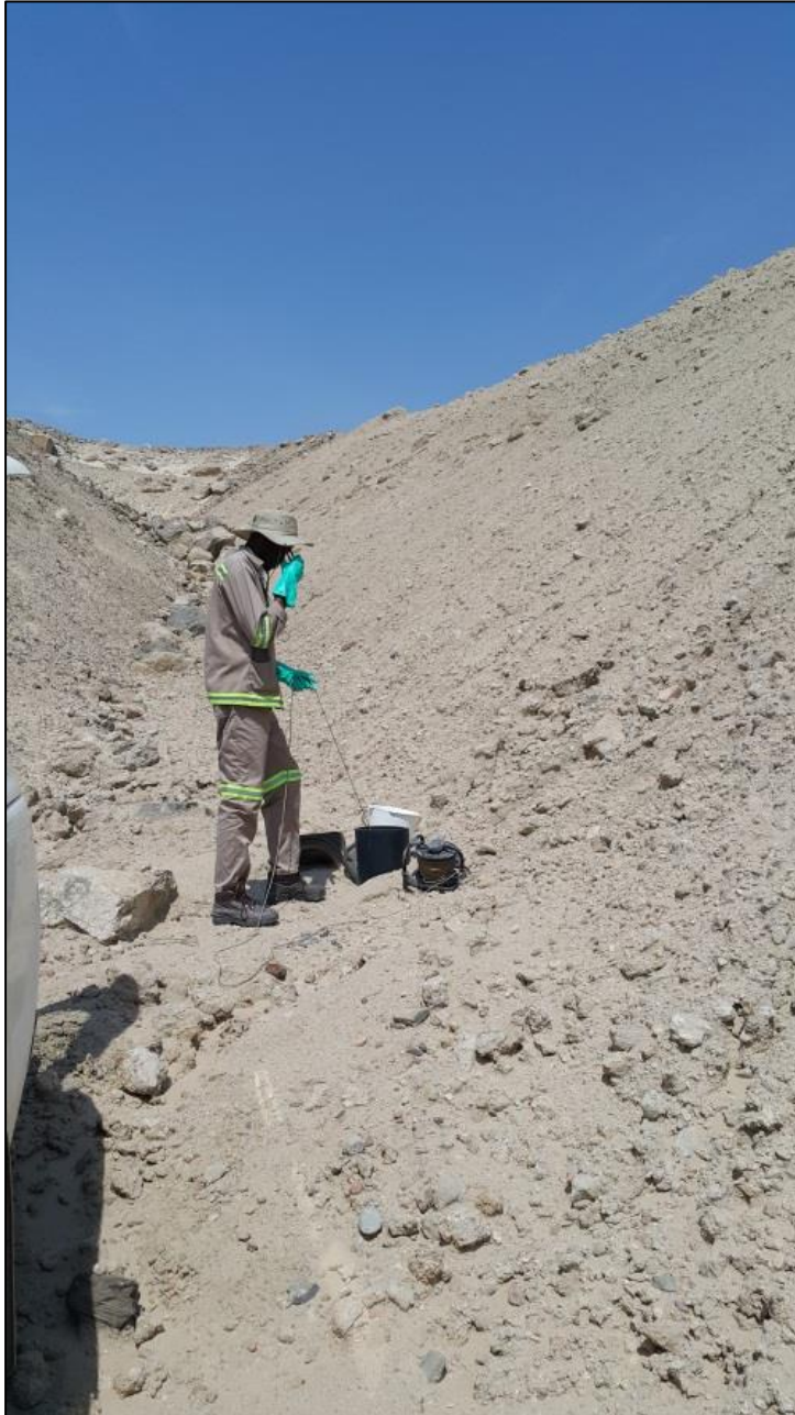
Figure 33. The LHU-1049 borehole directly below the unlined tailings
