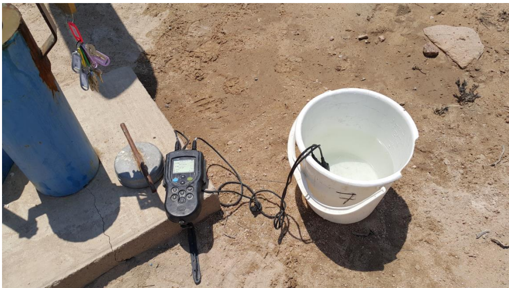
Figure 25. The Multi-parameter probe used to measure the onsite parameters in the field
