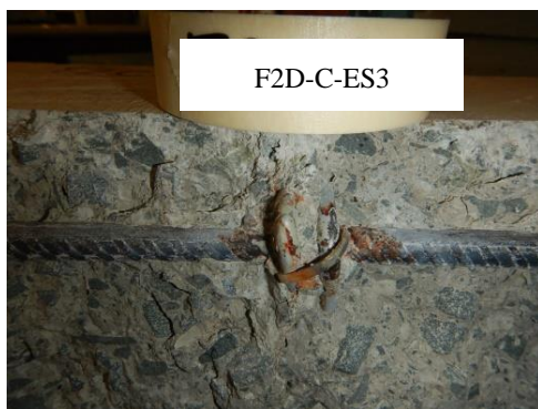
Figure E. 3: Photographs of corroded reinforcement bars in cracked PC/FA concrete (contd.)
