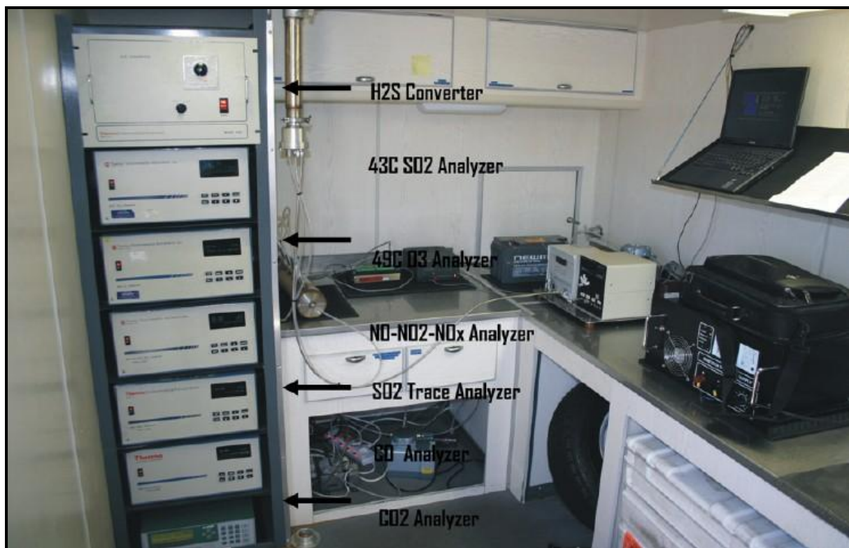
Figure 2.1 The ambient air quality monitoring station with a PC laptop logging data
