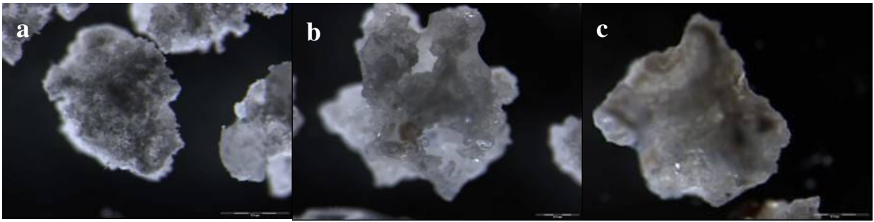
Figure 3.5: Stereomicrographs (darkfield, scale bar=1cm) of enterogranules: (a) uncoated at 40X (b) E L 100-coated at 25X and (c) E S 100-coated at 40X magnification
