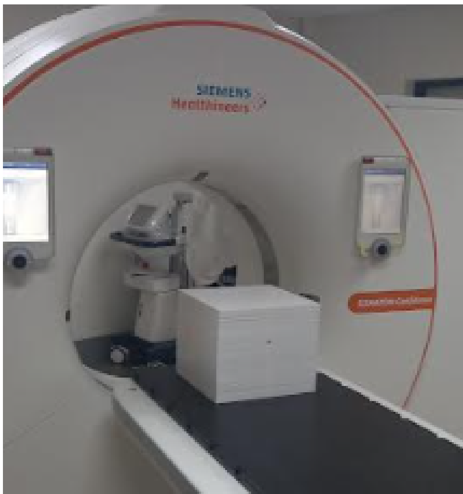
Figure 3.2: Photograph of a solid water phantom placed in a CT scanner for treatment planning and monitor unit calculation.
