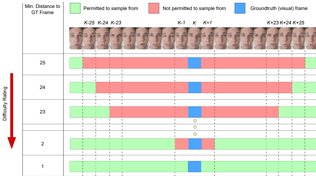
Figure 5.4: Visualization of the curriculum learning strategy we adopt by controlling the segment extracted from the input audio when producing out-of-sync videos with increasing difficulty.
