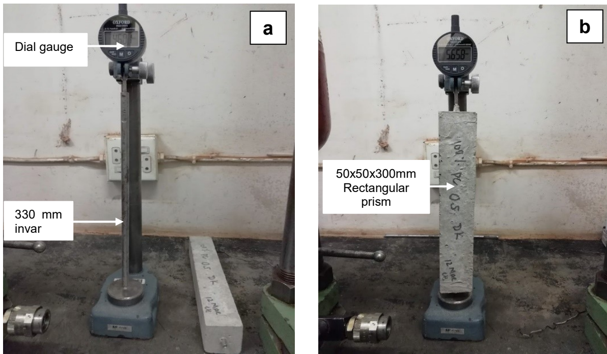
Figure 14: Photograph of length comparator a) to zero dial gauge b) measuring drying shrinkage
