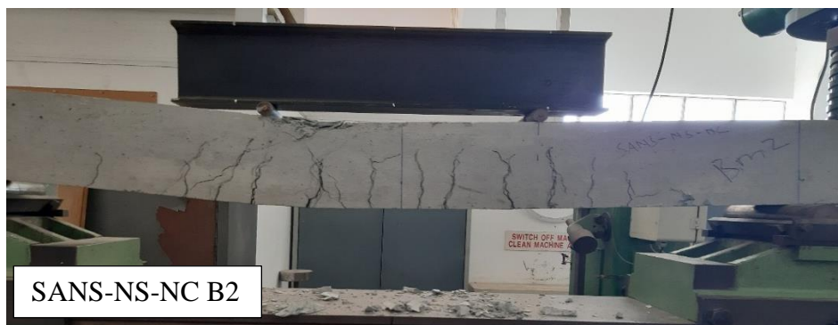
Figure 4. 10: Flexural crack pattern developed on SANS 10100-NS-NC beams
