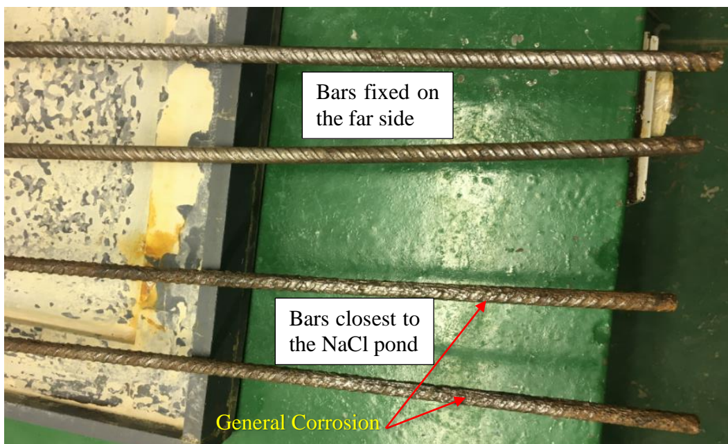
Figure 4. 5: Corrosion distribution on lap-spliced bars
