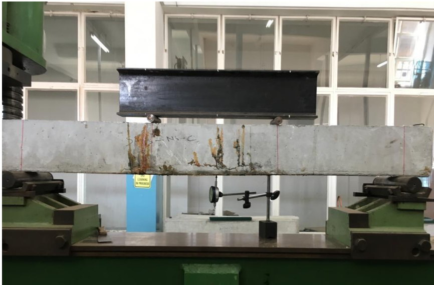
Figure 3. 10: Photograph showing support conditions and loading arrangement
