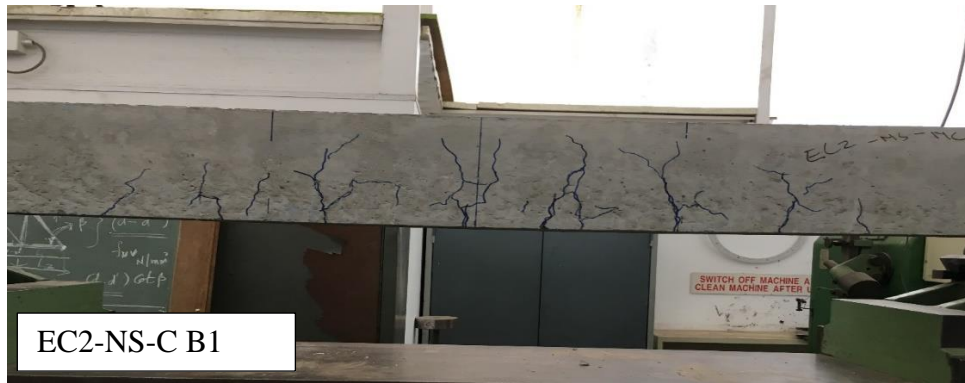
Figure 4. 12: Flexural crack pattern developed on EC2-NS-NC beams
