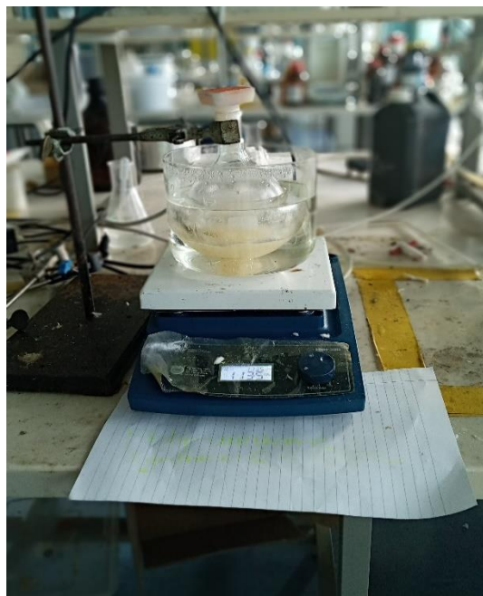
Figure 58: Epoxidation reaction set-up
