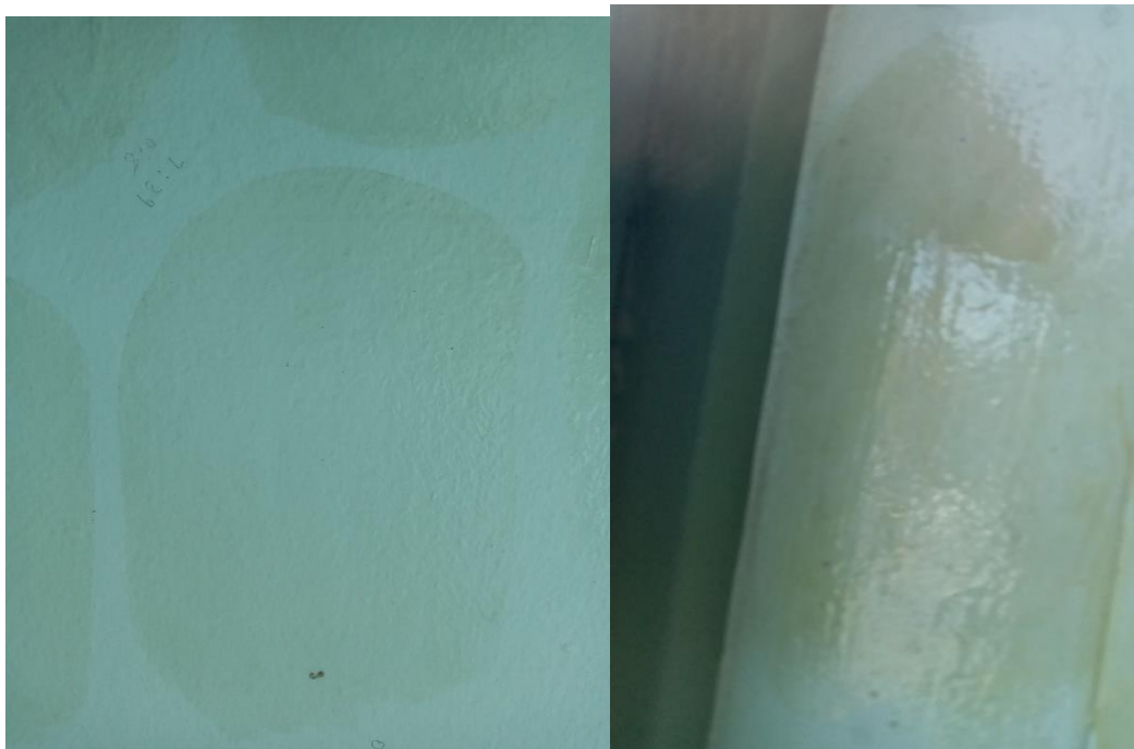
Figure 54: Polyurethanes based on CO and MDI without pigment after film formation
