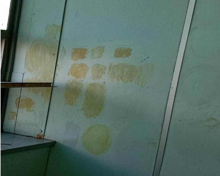
Figure 52: Picture of different samples painted on a wall to test for the drying time under atmospheric conditions.
