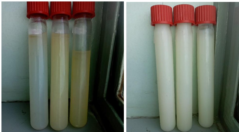
Figure 18: Representative samples of the PUs obtained from CO and RCO (left to right respectively)
