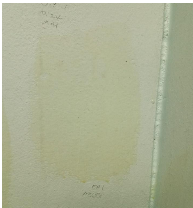
Figure 56: Epoxy resins with PA as hardener after film formation
