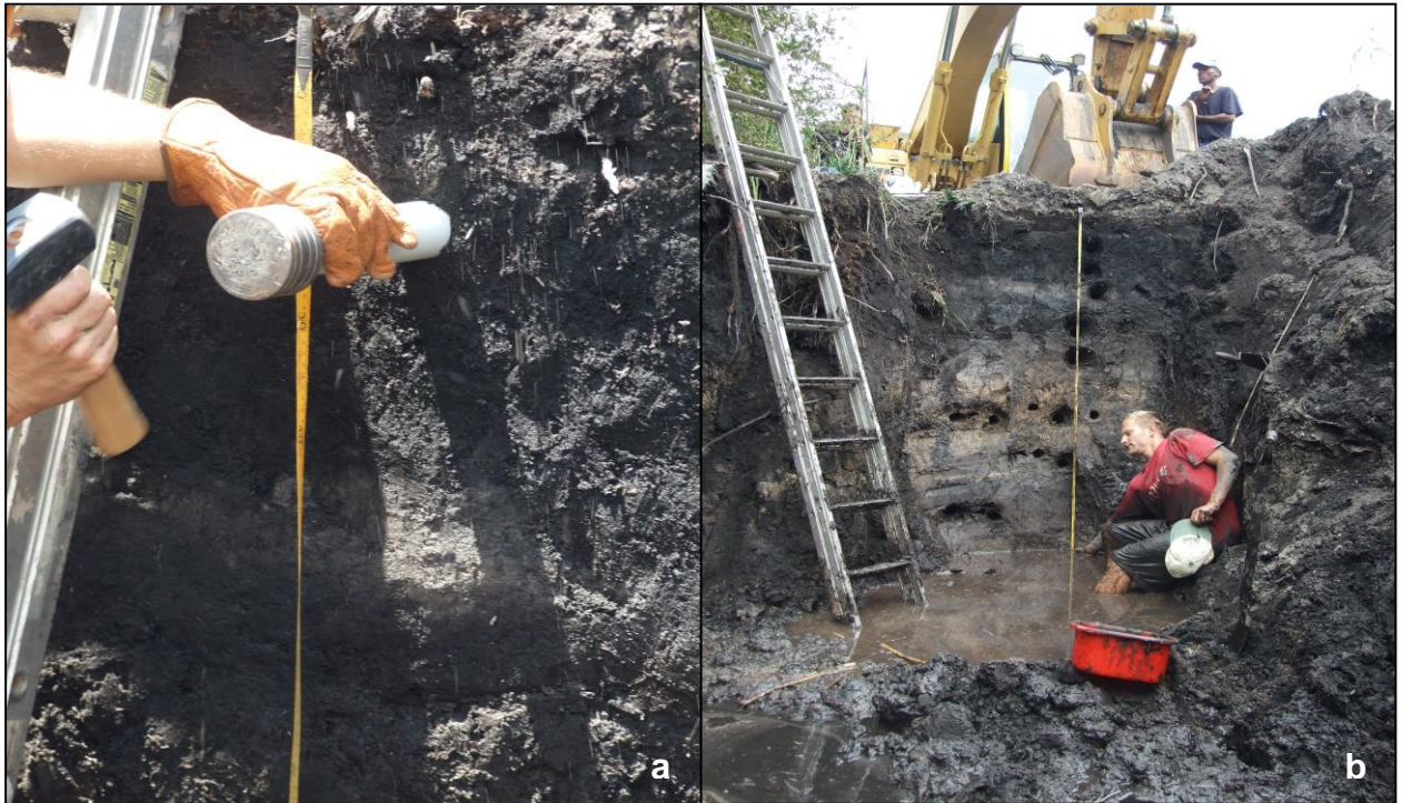
Fig. 4-3: a) Hammering in of OSL sample tubes into sand lenses of Pit C. b) Vertical measurement of sample depths from surface.
