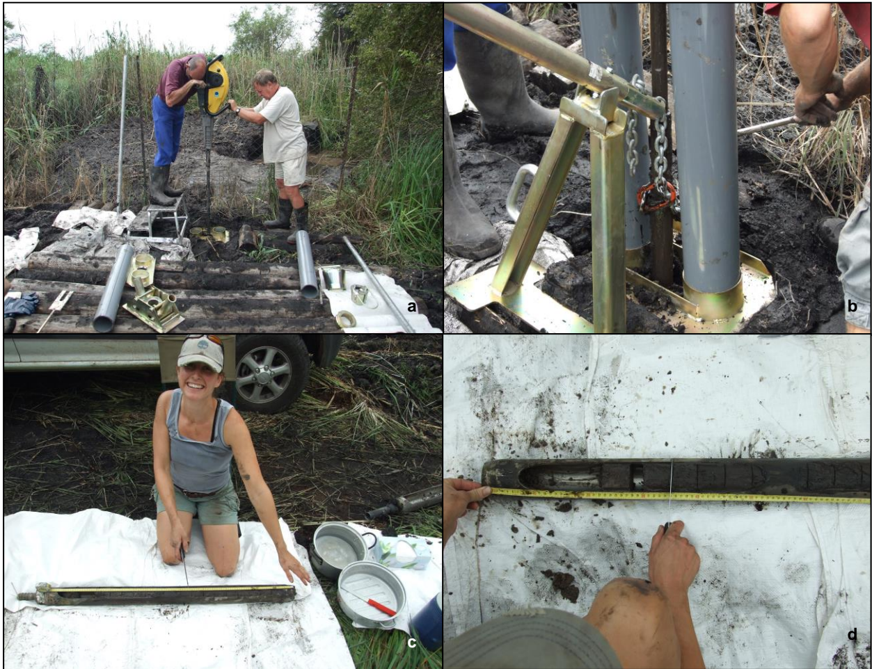
Fig. 4-4: a) Drilling of WK2 using a hand held percussion drill. b) Extraction of WK2. c) Onsite sample documentation and d) cutting of samples into 10cm intervals prior to packing.
