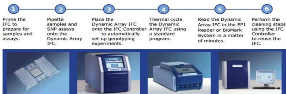
Figure 3.3: Fluidigm technique workflow ( http://www.incodom.kr/Fluidigm )
