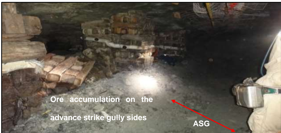
Figure 4.6 Ore accumulations on the advance strike gully side wall (Doornkop Shaft, 2017)
