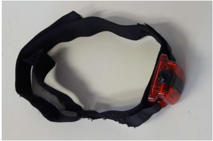
Figure 3.5 : The Actigraph Accelerometer on elastic band worn around the participant's waist.
