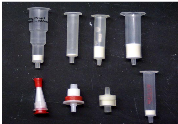
Figure 2.7: Types of SPE cartridges (Supelco, 1998)
