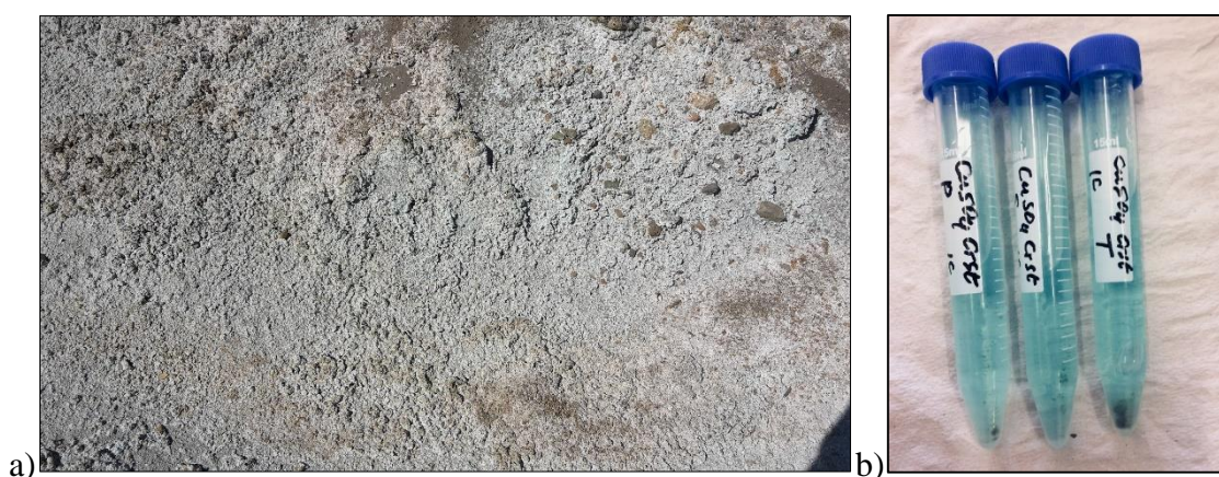
Figure 5.10: a) Copper crusts in the field; b) Intense blue colour of leachates obtained from Copper crusts sample
