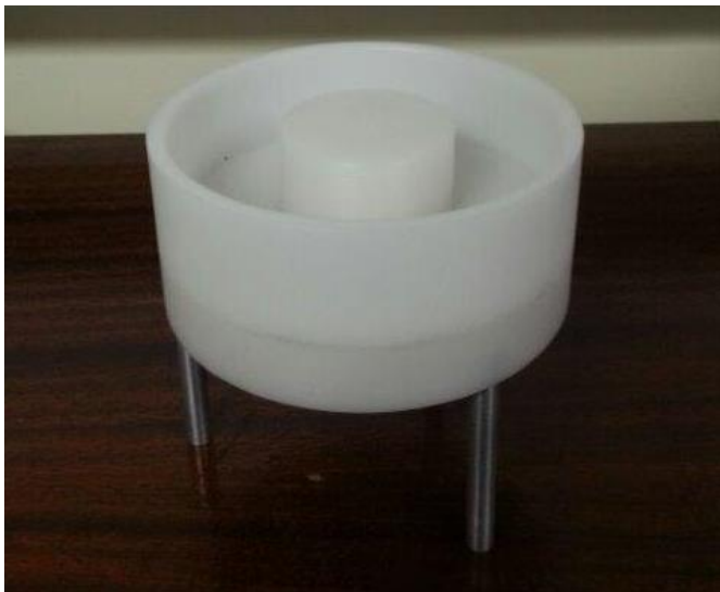
Figure 3.3: Doughnut shaped irradiation jig used during pupal irradiations
