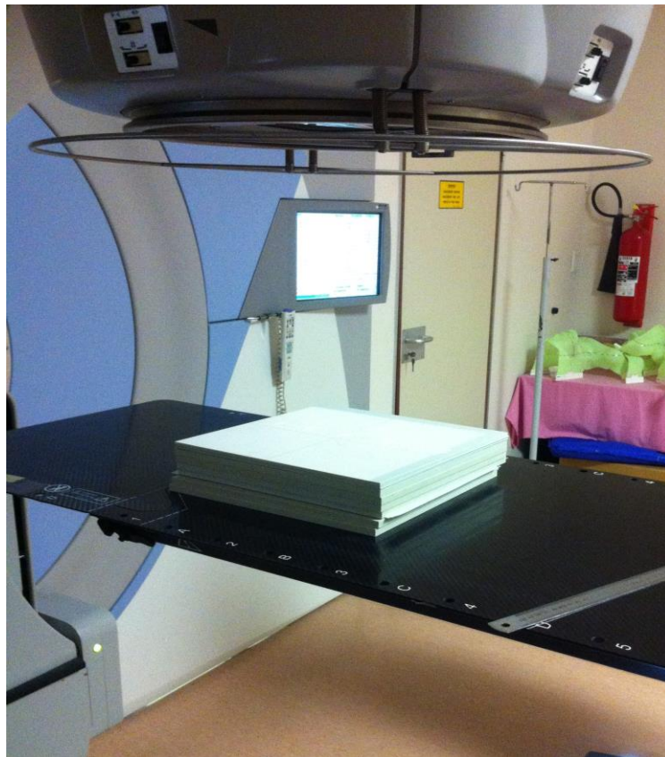
Figure 4.9: The positioning of the Polystyrene phantom for exposure of films at the isocentre of the LH Linac
