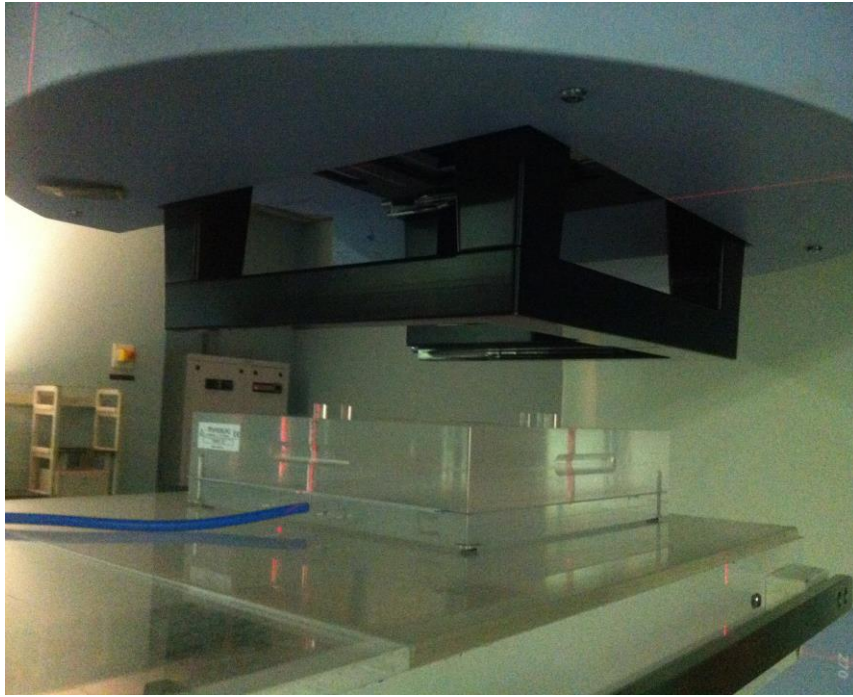
Figure 4.8: The positioning of the UIP for the exposure of films at the SSD 63 cm setup for the CMJAH Linac.
