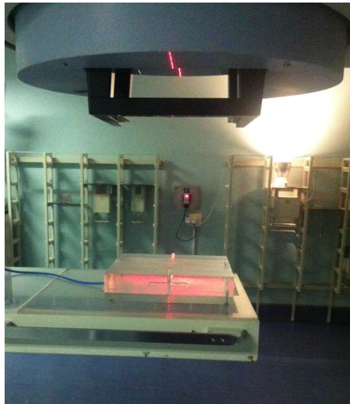
Figure 4.7: The positioning of the UIP for the exposure of films at the isocentre of the CMJAH Linac.
