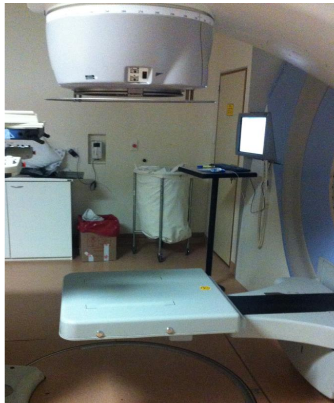
Figure 4.11: The position of the EPID for the exposure of EPID images for the LH Linac.
