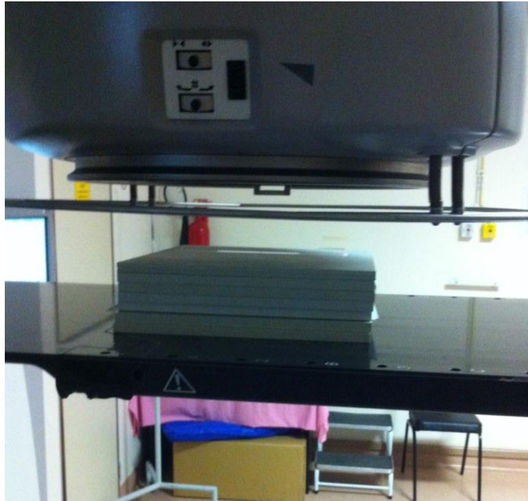
Figure 4.10: The positioning of the Polystyrene phantom for the exposure of the films at the SSD 63 cm setup for LH Linac.
