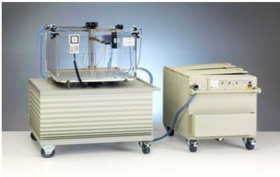
Figure 4.12: The PTW MP3 water tank, support table and reservoir tank used with the LA 48 at CMJAH.
