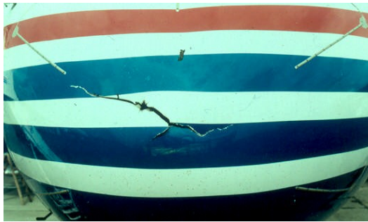
Figure 2.5: Photograph: Aircraft nose radome punctured by lightning (American Airlines photo).
