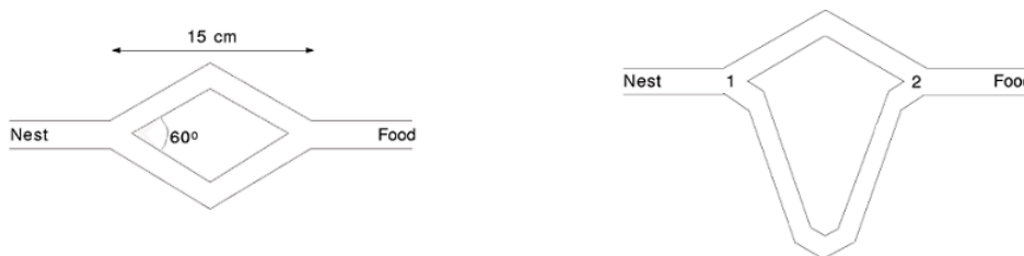
FIGURE 4.1: Experimental setup for the double bridge experiment. (a) The left image has equal branch lengths. (b) The right image has different branch lengths. ([28], 2004, p.3)
