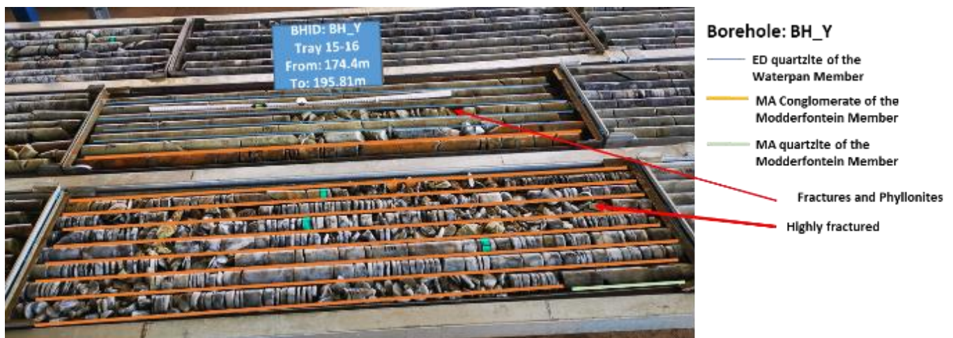
Figure 5-6: BH_Y core illustrating diced core, faults, and joints that can allow the flow of water and is associated with sample SD2
