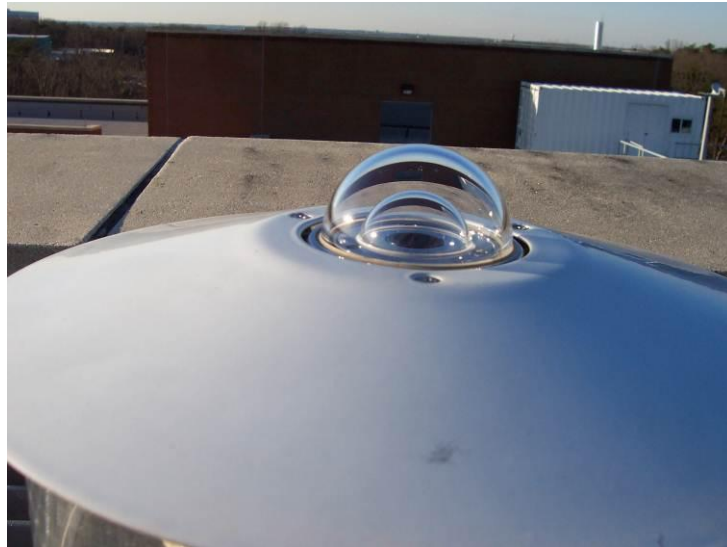
Plate 1-1 Precision Spectral Pyranometer (PSP) showing the dome (external glass) and the case (internal glass) covering the sensor.
