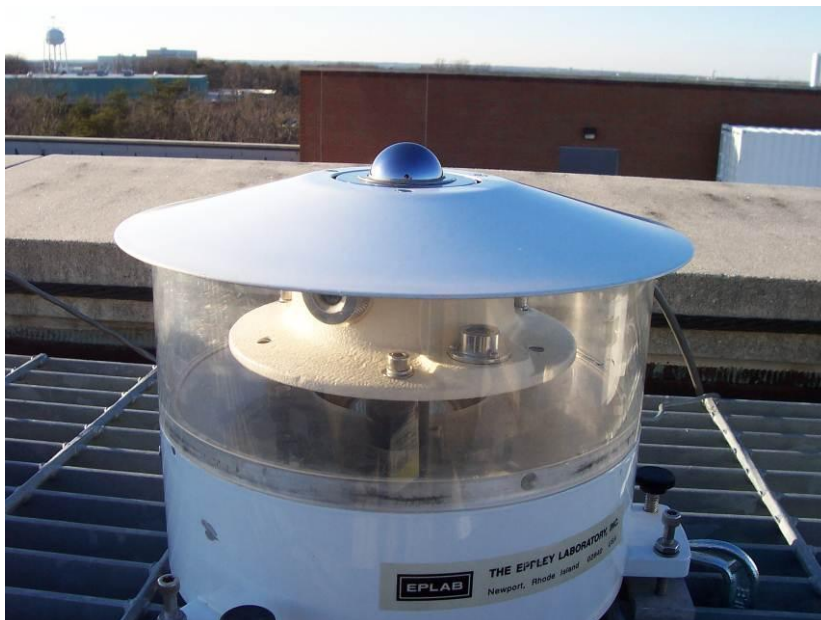
Plate 1-2 Precision Infrared Pyranometer (PIR), manufactured by Eppley Laboratories.
