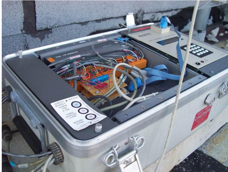
Plate 1-3 The CR7 data logger used during solar radiation measurements at Skukuza site during SAFARI 2000 field experiment (September 2000).
