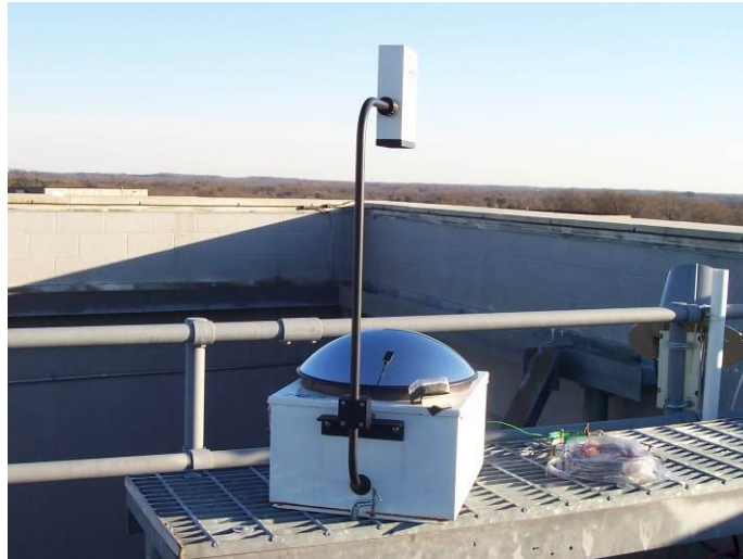
Plate 1-4 Total Sky Imager (in the mounted position) at Goddard site (January 2004).
