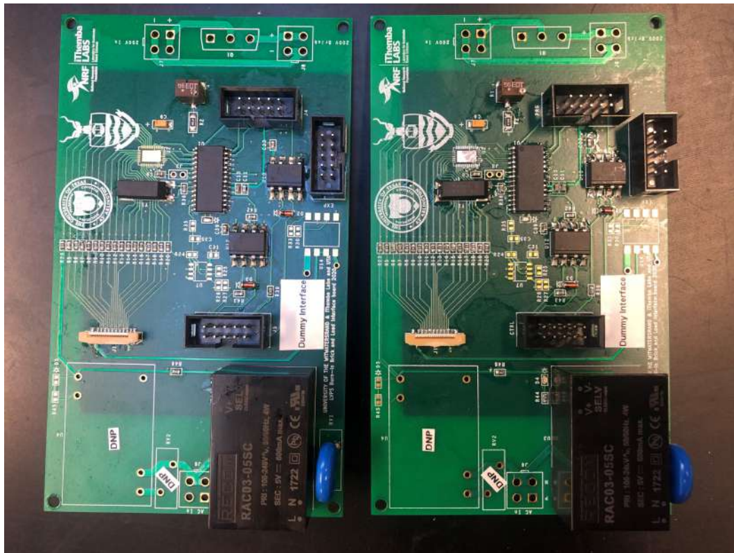
FIGURE 5.4: Two Burn-in test station dummy load interface.
