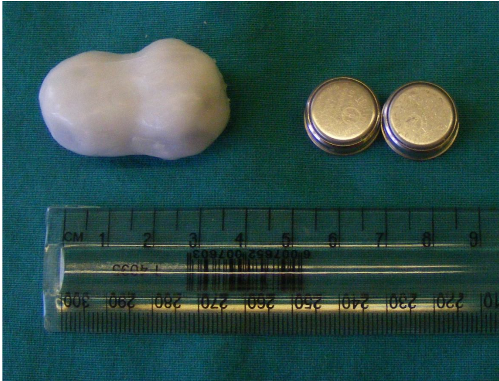
Figure 2.2. The typical size of the iButton miniature data logger unit, waxed (left) and unwaxed (right), which measured subcutaneous body temperature.
