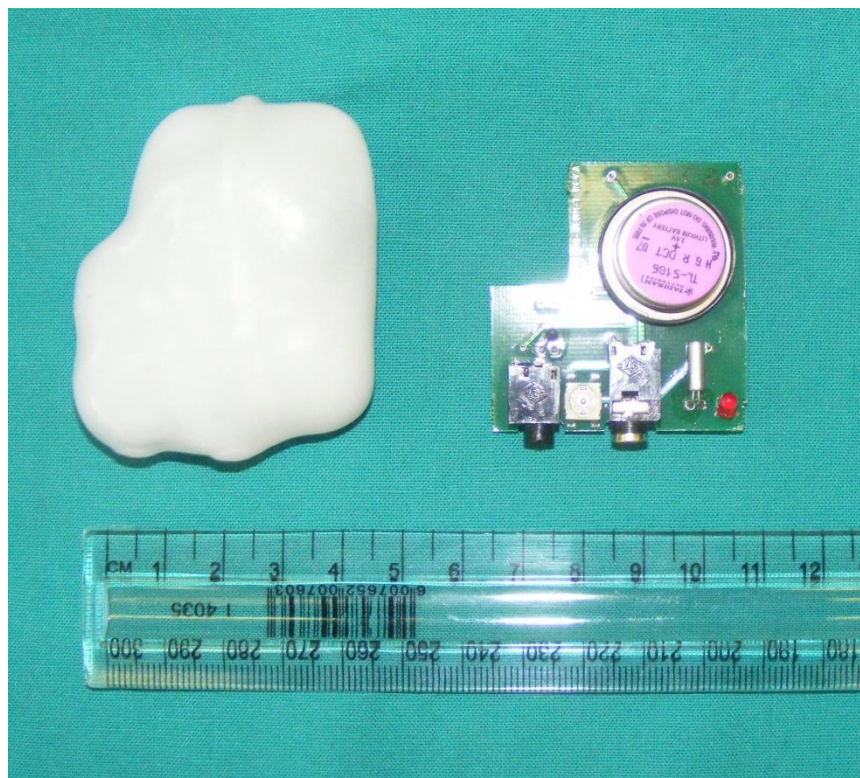
Figure 2.1 The typical size of the Stowaway miniature data logger, waxed (left) and unwaxed (right), which measured core body temperature intra-abdominally.
