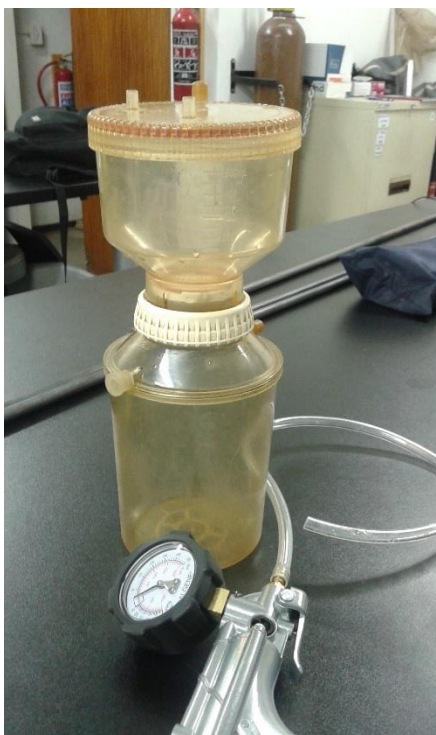
Figure 5 Filter rig and pump.
