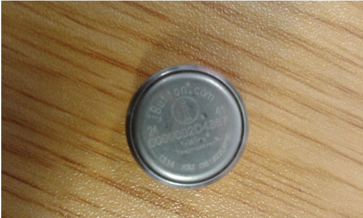
Figure 9 The iButton data loggers that were used to monitor stream water temperature during the year of monitoring.
