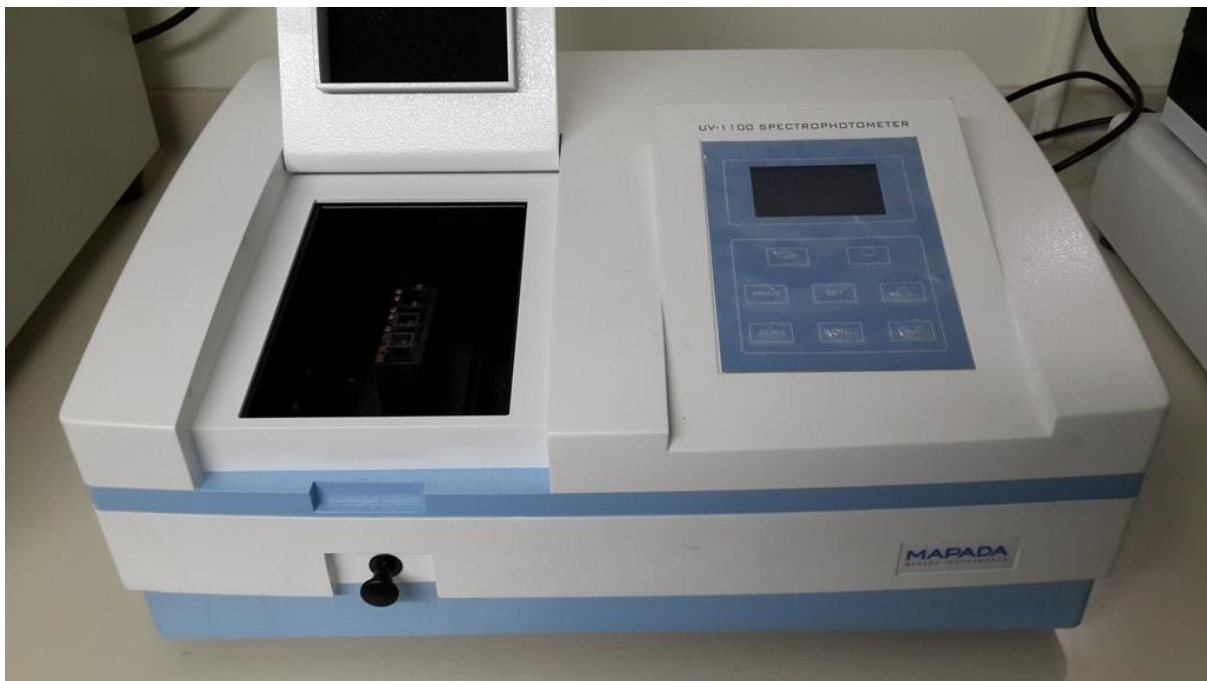
Figure 10 Mapada UV-1100 spectrophotometer used for spectral absorbance analyses.
