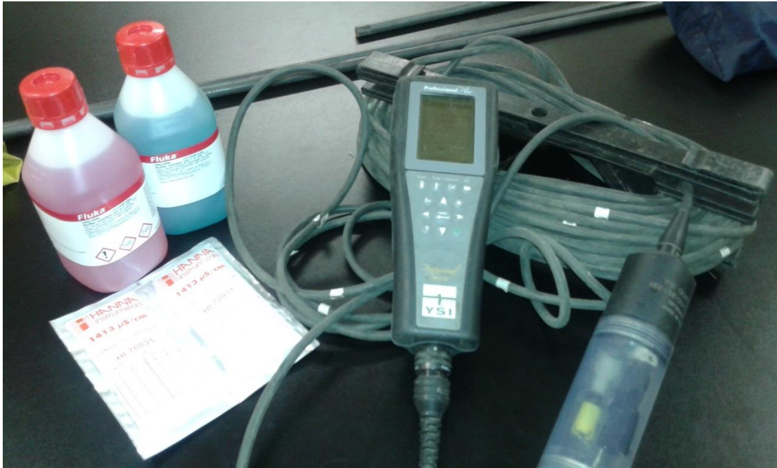
Figure 8 The YSI Multiparameter probe used to collect field measurements; and the standard solutions (pH and conductivity) that were used to calibrate it.
