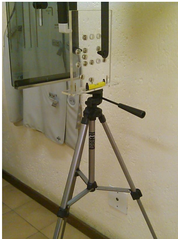
Figure 3.3 The perspex sheet with embedded stainless steel balls, held vertically upon a horizontal support, as confirmed by a spirit level.
