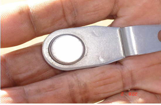
Figure 4: Prepaid water meter Tag
