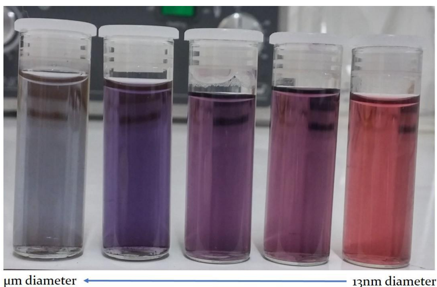
Figure 3.9: Effects of AuNP Size on Nanoparticle Solution Colour. AuNP synthesis yielded very distinct colour differences as the size of the nanoparticles was increased. As the nanoparticles became larger, the solution underwent a blue shift. A gold tinge is also present in the far-left vial.
