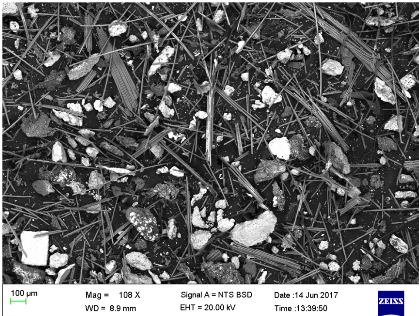
Figure 4.12 SEM image of the magnetic separation residue magnified by a factor of X108
