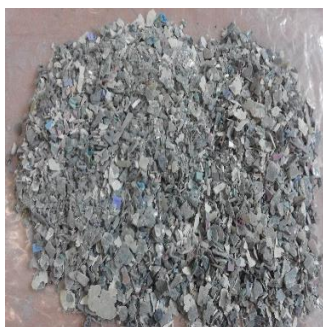
Figure 4.5 Crushed dismantled circuit boards -10mm
