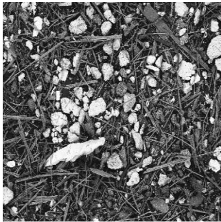
Figure 4.7 SEM image of the pulverised e-waste DESCO sample enlarged by a factor of X108
