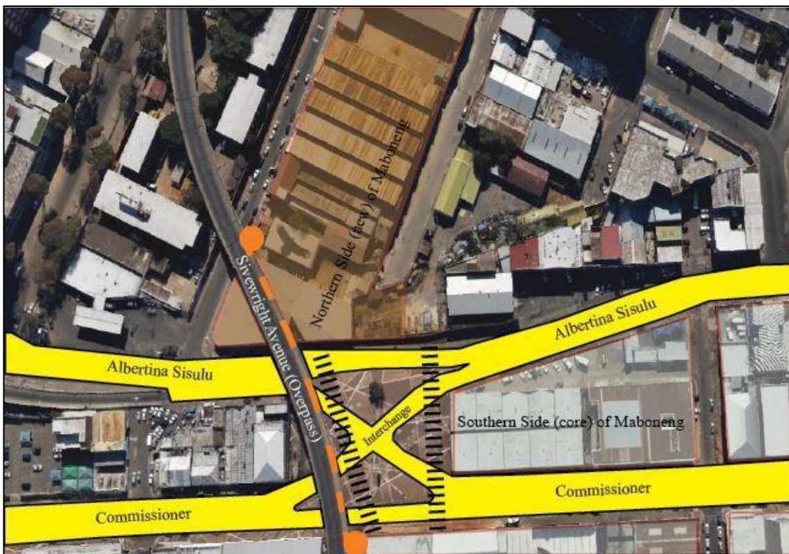
Figure 33: Map illustrating the poor pedestrian movement channels across Albertina Sisulu and Commissioner Streets interchange (Hashed black lines) and the proposal for new 'hanging' pedestrian bridge under the overpass (Orange dashed lines with circles). (Source: Rory Murtagh, 2015).
