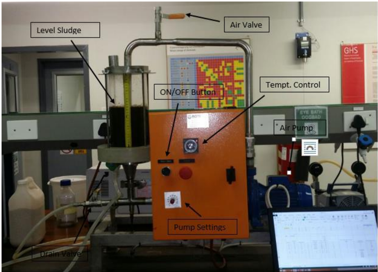
Figure 4.1: The dynamic foam rise test equipment for batch experiments
