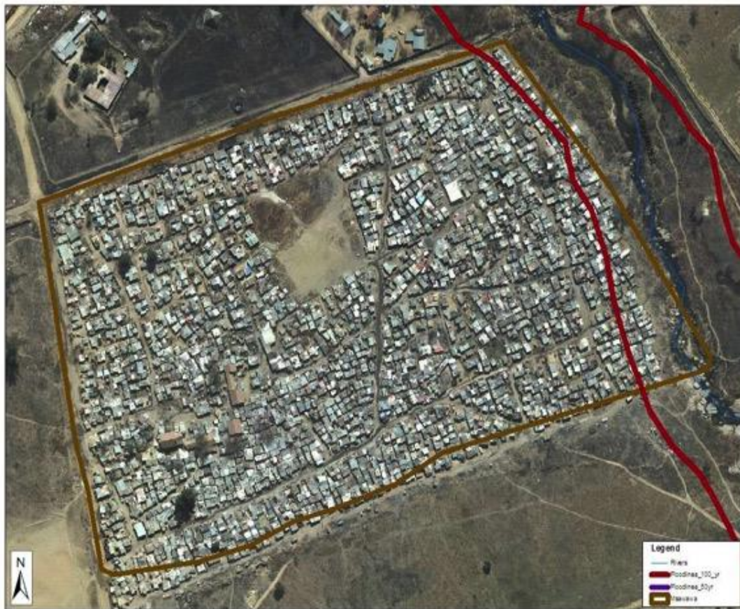
Figure 4.8: Map of Msawawa showing the flood line in red and the routes that act as a form of drainage in the settlement, those closer to the river being eroded into gullies (CoJ, 2014c)
