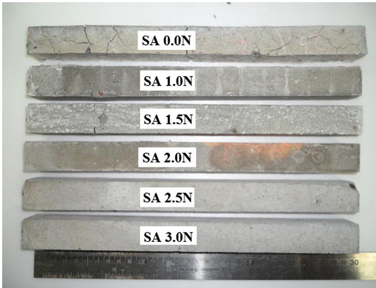
Figure 2-8: Concrete mixtures made with BOF-S that had been chelated with oxalic acid after four days steam curing process [photograph by Ding (2017)]
