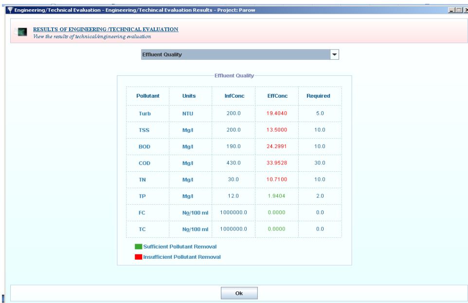
Figure 6.14(b): Dialog screen showing effluent quality result of the Parow WWTW when treatment units are operating at average pollutant removal efficiency
